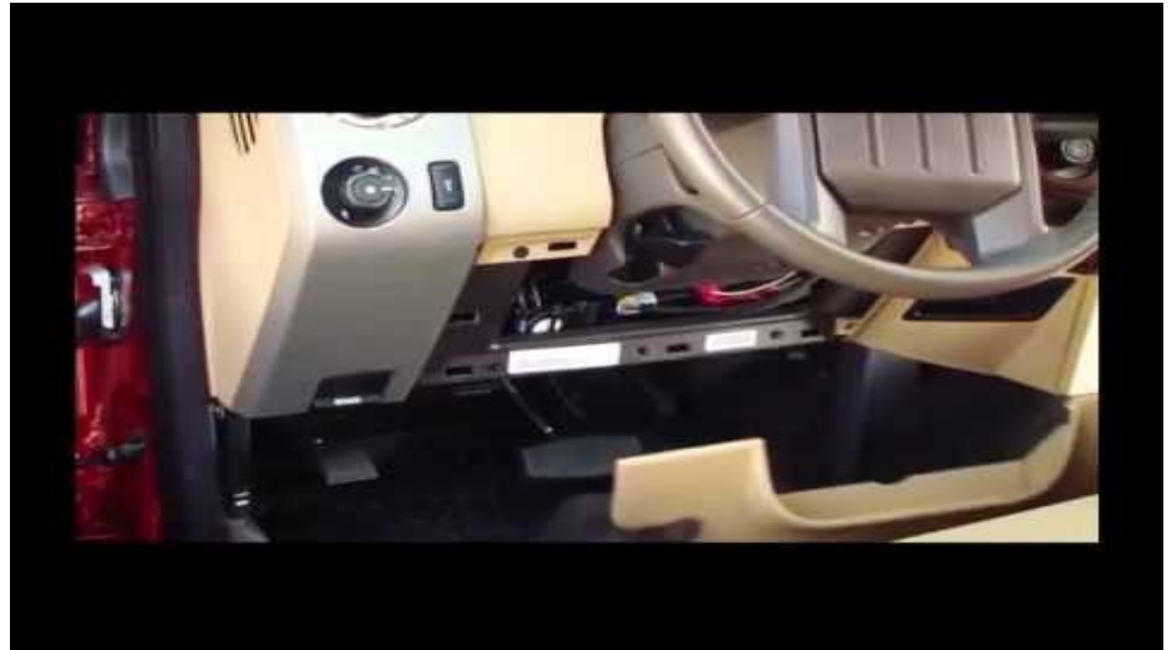
Installing the Y-Harness
